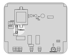
The electronic control system is protected by a 0.16A fine-wire fuse on the PCB in the inside of the device. The short-circuit protection for the filter pump must be provided by a backup fuse of maximum 16A on site.
