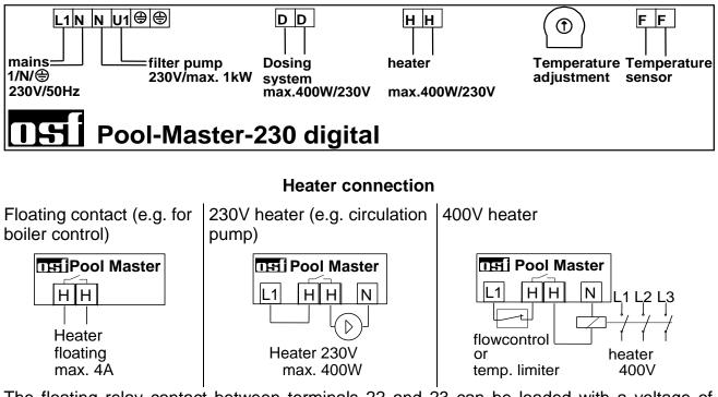
The floating relay contact between terminals 22 and 23 can be loaded with a voltage of maximum 230 V and a current of maximum 4 A.
