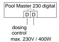
There is a floating relay contact between terminals D-D. This can, for example, be used for activation of the dosing system (the contact remains closed during filter operation).
